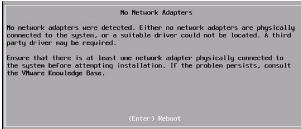
Figure 6. No network adapter error during ESXi installation
